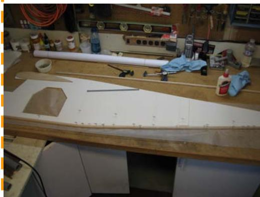
The build started with the fuselage. Unfortunately I did not take as many pictures with the build of the Beaver as I did with the Duck, but there are a couple of shots of the fuselage. As you can see the side is built on the 5 mm foam board with all the framing glued onto the inside of the foam board.
