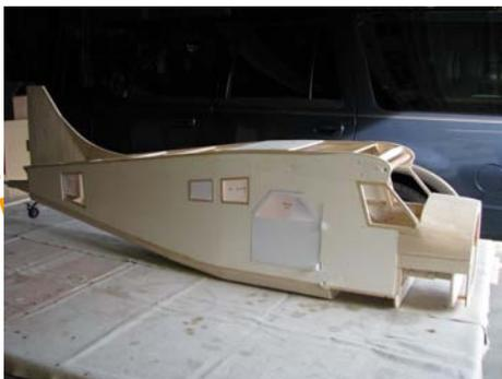
by taking off the prop and unfastening 6 cam-lock fasteners. The kit came with music wire for the landing gear which I did not like. I ordered aluminum gear from TNT. Yes, that too added weight. It weighed three pounds. I cut a couple of lightning holes in it where it attaches to the bottom of the fuselage, which eliminated about 0.4 pounds. The completed model weighs in at 44 pounds. The wheels and landing gear account for 4.5 pounds and the engine 12.5 pounds.
