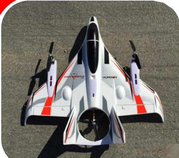
Augie Caresani's CONVERGENCE, a different concept from Horizon Hobbies. Yes, it has three propellers, two which are tilt rotor technology. It is fast. Obviously when in forward flight (front engines horizontal) the rear rotor (propeller) is not engaged. Augie says the takeoff and level flight are the easy parts, but transitioning from forward flight to hovering mode is problematic. It has no landing gear so a hovering type landing is a necessity.
