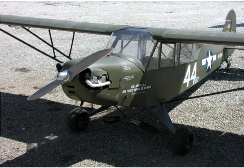
Also seen at the memorial fly-in was this 1:3 scale Piper Cub L-4 finished in Air Force colors. It features a four cylinder, four stroke O.S. 240. Surprisingly quiet, the plane flew very scale like.
